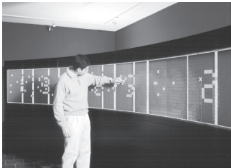
Fig. 4. The BioWatch application on the BioWall, 2002. (© Daniel Mange. Photo © Corine Sporer.) In the BioWatch application, the visitor can inject faults in the electronic substrate and observe the machine repairing itself.
