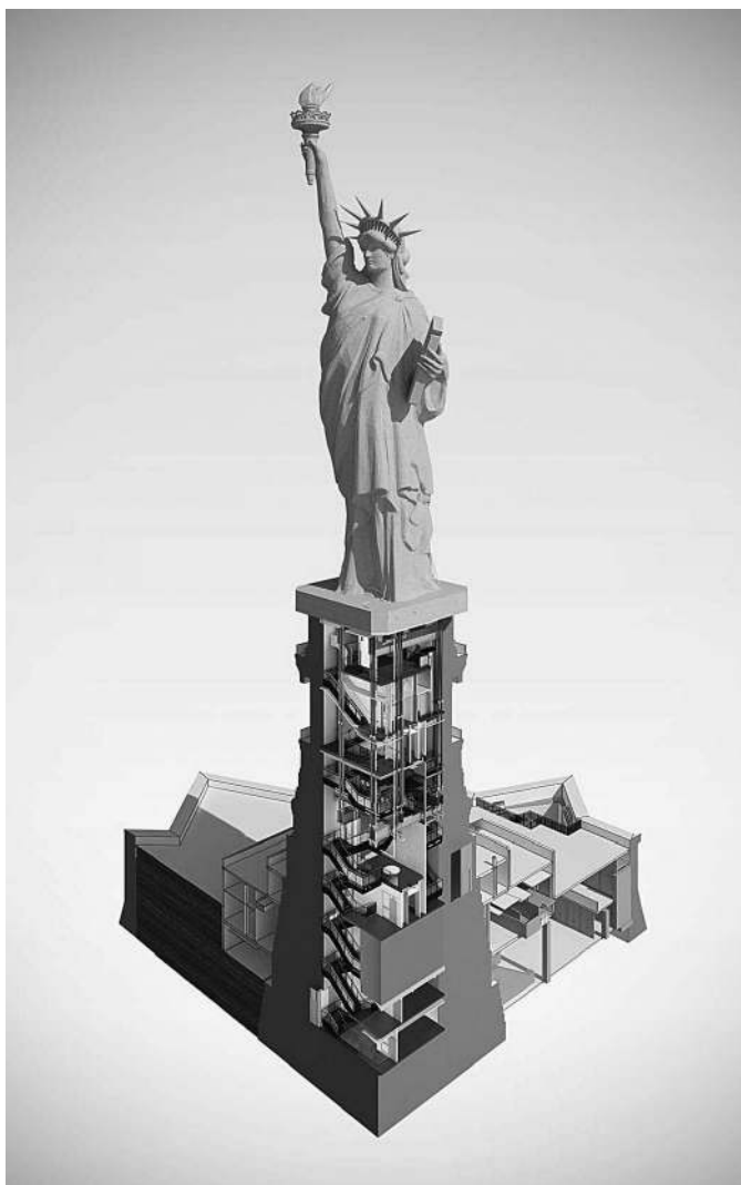
Figure 5. Cutaway view showing the two new stairs in the pedestal. Image by author
